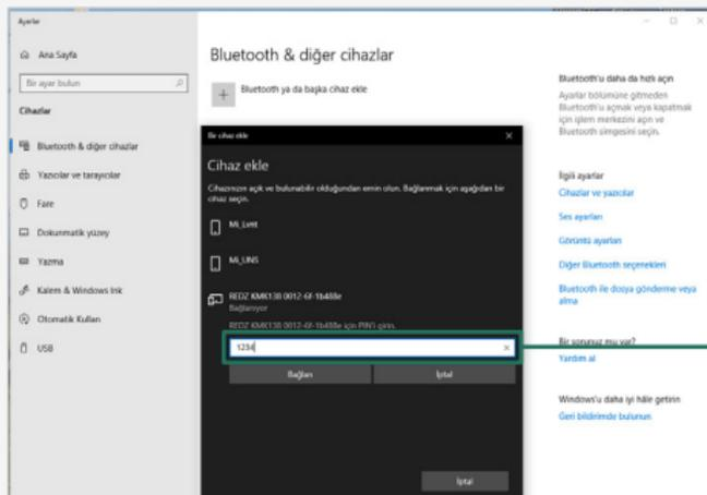
Enter the pin number «1234» to complete pairing the probe with your PC.
