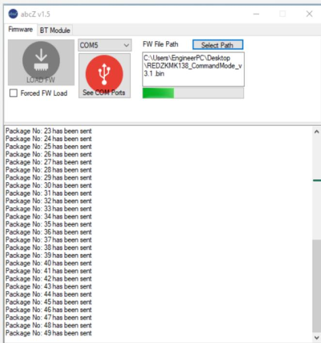
The firmware upgrade process will be shown on the window of the software.
