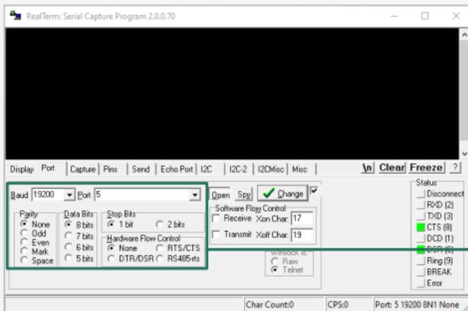
Select the serial settings and COM port. The correct outgoing COM port of the probe should be selected and the serial settings should be 19200 baud rate with 8N1 data type.
