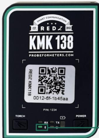
When you connect the probe with abcZ software and upgrade process starts the Bluetooth led will be on.
